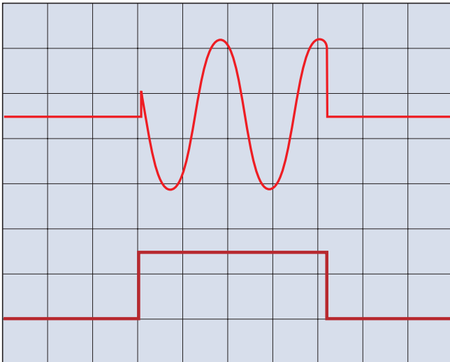
Figure 3: Output signal controlled by a GATE signal
